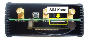
3. Pull out the preinstalled mdex SIM card and insert your SIM card into the SIM card slot according to the picture.
