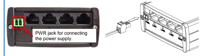
The MX510 can be alternatively supplied with another power supply (7V - 30V DC). In this case please remove the power adapter cables from the green connector (loosen the screws) and connect the cables from your own power supply.
